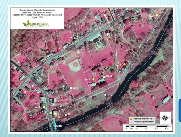
"NRCS and MWA are committed to assessing the changes in ground water that occur as a result of the project and any resulting impacts to domestic water supply wells. This assessment will involve installing monitoring points and measuring ground water levels near the river and in selected wells prior to and subsequent to removal of the dam. "
